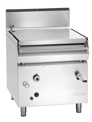
The 900 series tilting frying pan in the well-known premium stainless steel design. The crucible is made entirely of stainless steel and has a 70 litre capacity. The gas model with manual tilting device has a water inlet tap and is designed for a cold or hot water connection.
