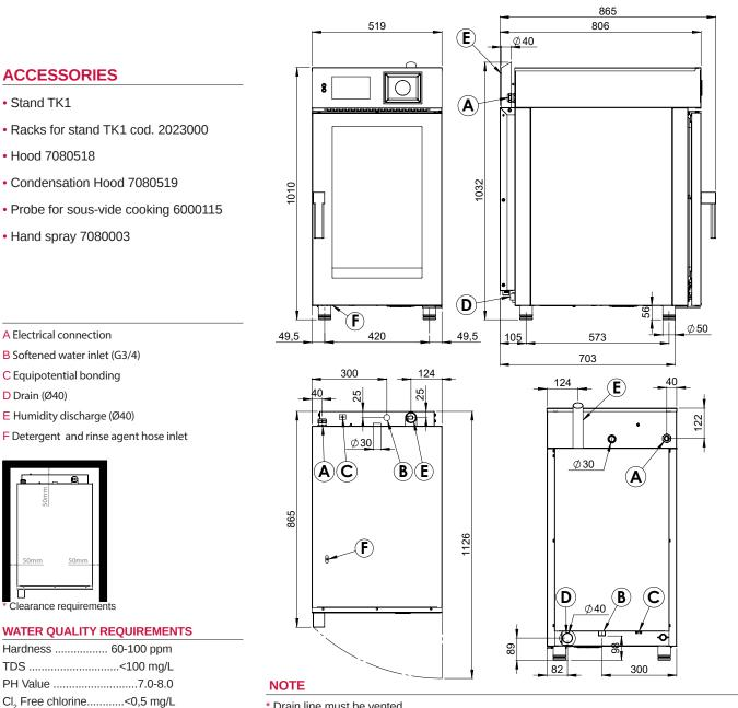
\* Drain line must be vented
