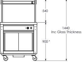
\*800mm high units also available, overall height and tray slide height reduce by 100mm accordingly
