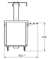
\*\* Unit depth is 757mm with the tray slide down All dimensions in mm
